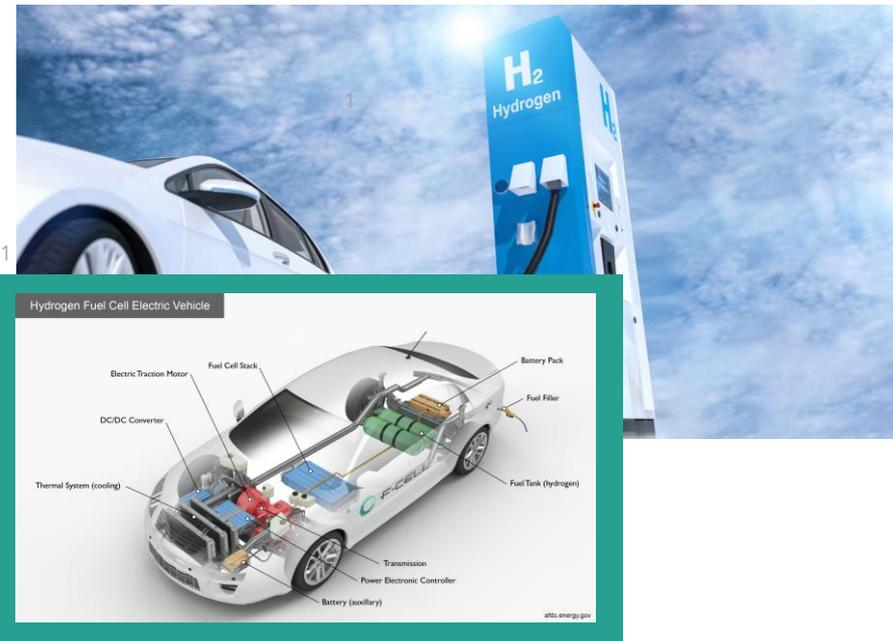
1) *How Do Fuel Cell Electric Vehicles Work Using Hydrogen?*
